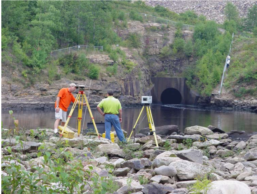
Figure 10-13. Optech Iris Unit positioned in center of river bed at the Francis E. Walter Dam site located in Whitehaven, Pennsylvania.
