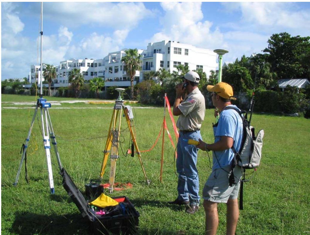
Figure 2-7. RTK base station and radio link transmitter--and rover with backpack (Key West Harbor Dredging Project 2004--C&C Technologies, Inc. & Jacksonville District)
