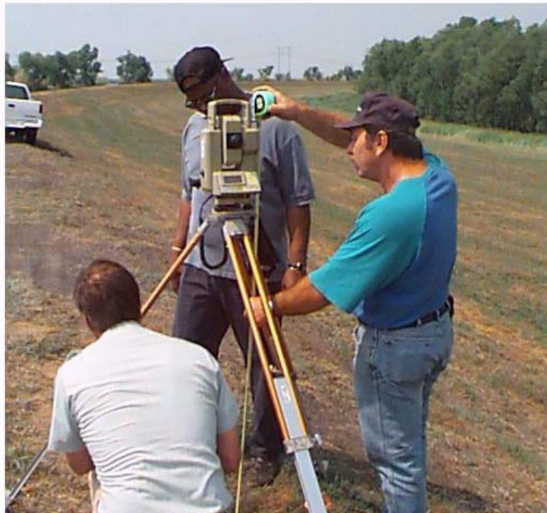
Figure 8-1. Wild TC-1010 Total Station with TDS-HP48GX Data Collector 1998 Levee Survey at Bayou Segnette (New Orleans District)
