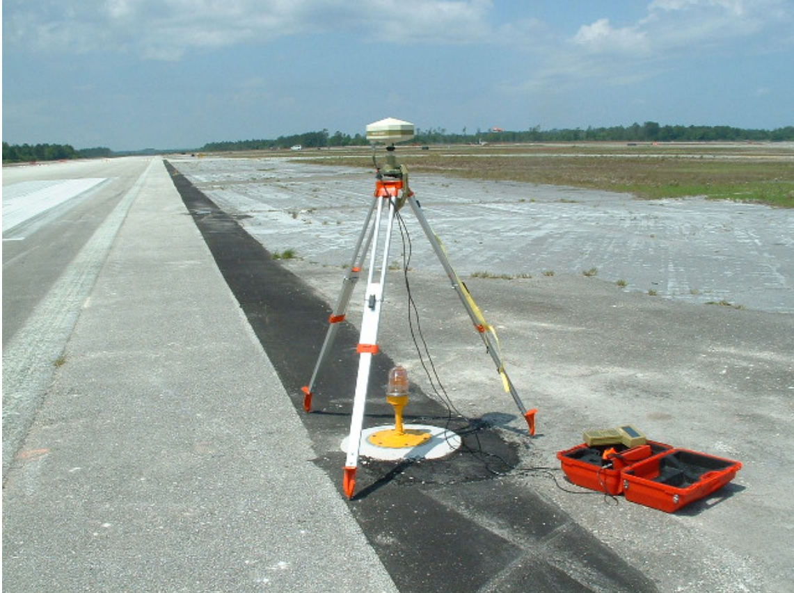
Figure 2-3. Airfield NAVAID positioning using Fast-Static GPS methods
