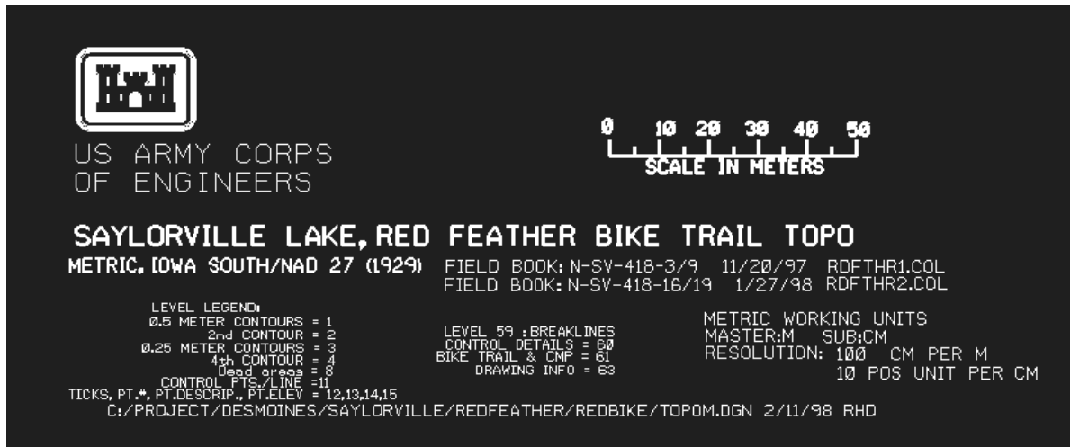
Figure F-2. Title block and legend from final drawing depicting level assignments in dgn file
