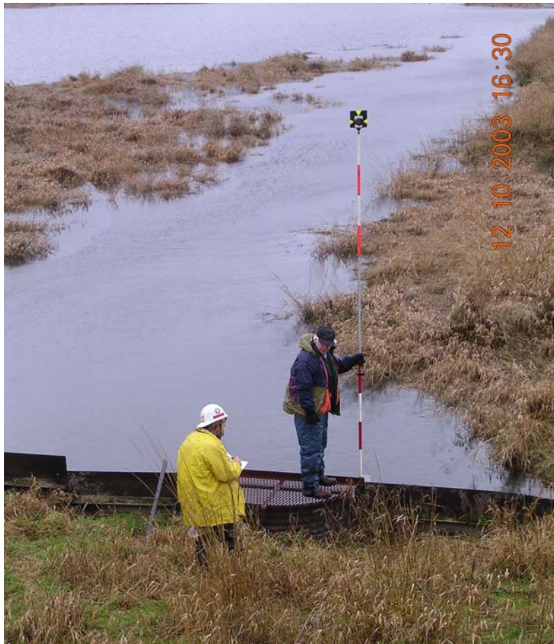
Figure 8-4. Prism pole (Portland District)
