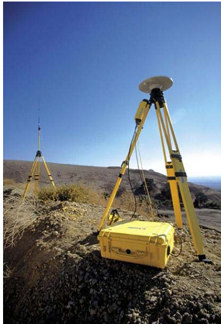
Reference (Base) Station
