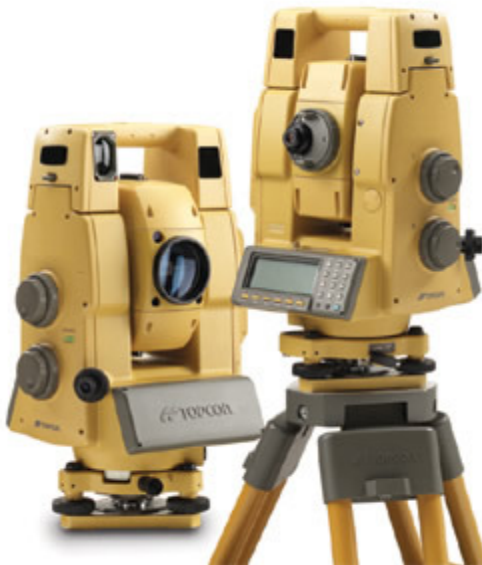
Figure 8-5. TOPCON GPT-8200 Series Reflecterless-Robotic Total Station can make reflectorless measurements out to 4,000 ft and prism measurements to 23,000 ft
